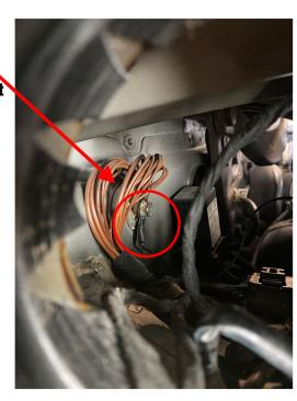
To supply the control unit with power, the red cable must be connected to ignition plus (terminal 15).
