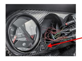
Open the instruments and replace the windscreen wiper switch (if fitted) with the supplied switch.
