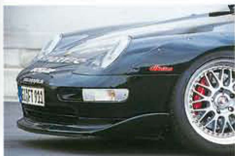
Record-breaking car began life as a relatively ordinary 1996 911 Carrera RS, although front and rear body mods (above and left) make it look more like a 911 GT. The all-wheel-drive transmission system was taken from a 911 Turbo 4. Wheels (left) are three-piece Cargraphic Racing items; see text for details
