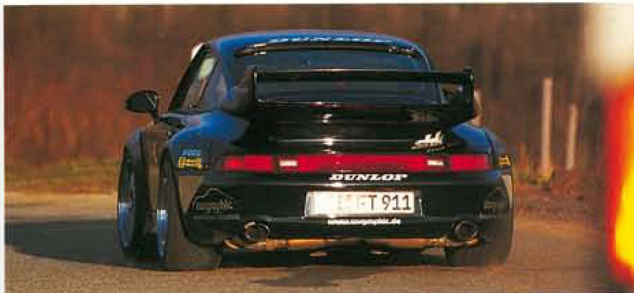
Record-breaking car began life as a relatively ordinary 1996 911 Carrera RS, although front and rear body mods (above and left) make it look more like a 911 GT. The all-wheel-drive transmission system was taken from a 911 Turbo 4. Wheels (left) are three-piece Cargraphic Racing items; see text for details
